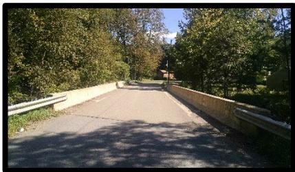
**[BMS 08-7238-0698-0000]** Fall Run Road (T-598) over Johnsons Creek: This structure is located on Fall Run Road 0.2 miles south of S.R. 467. The structure is a prestressed concrete/multiple box beam, built in 1991. The span length is 87 feet and a width of 22 feet. The last inspection report dated July 22, 2015 indicates the overall condition of the structure as good. The structure has no posting restrictions and is inspected on a two year (24 month) frequency.
